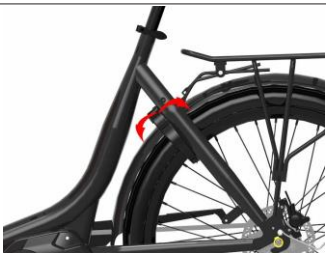
Image 29: Rotate the key 20 to 30 degrees clockwise
