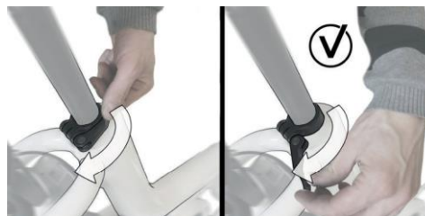
Image 6: Opening the seat post quick release
